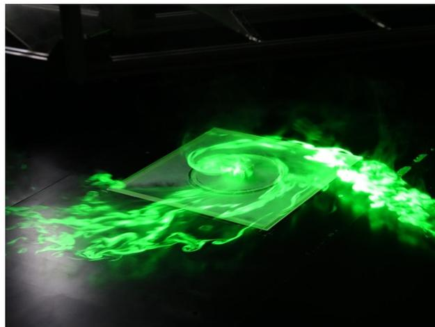
Figure: Flow visualization depicting tornado like flow in presence of building model
